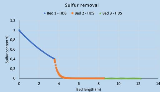
Figure 3. The sulphur removal along 3 HDS reactor beds
