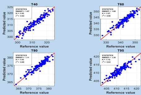
Figure 2. Estimation of feed properties based on NIR measurements
