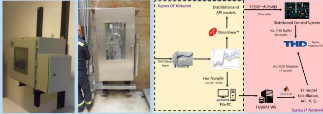
Figure 1. Online NIR analyser and preconditioning system (left) and IT/OT integration structure (right)
