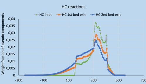
Figure 4. Cracking reactions along 2 HC reactor beds
