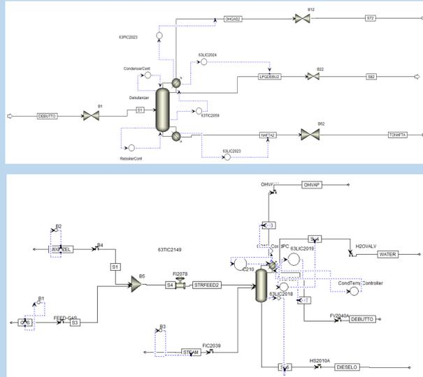
Figure 5. Separation model in Aspen HYSYS
