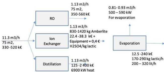
Figure 4. Detailed downstream processing analysis
