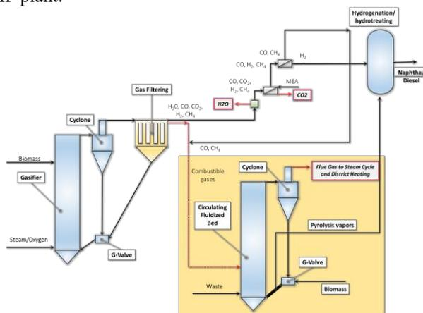
Figure 1: Process scheme with pyrolysis integrated with CHP G-valve and gasifier integration at the upfront of CHP plant (highlighted portion shows the existing boiler of CHP plant)
