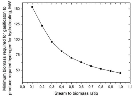
Figure 2: Effect of steam to biomass ratio on the minimum gasification capacity requirement to produce the hydrogen needed in hydrotreating
